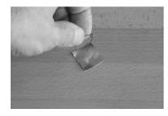
Cut a 20mm square of metal Duct Tape.
